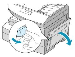
**4** Carefully remove the misfeed paper in the direction shown.
